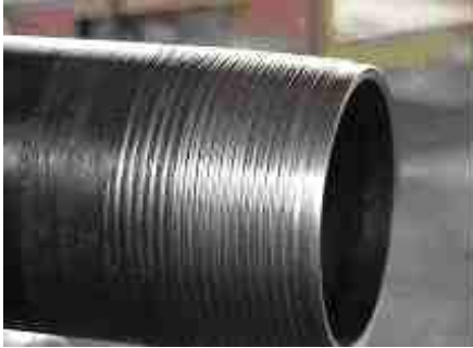
Figure 1. Dopefree coated pin end (4"1/2)
