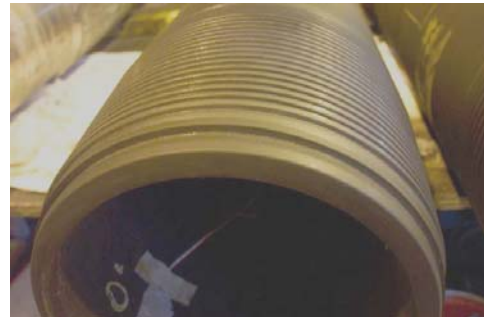
Figure 10. 7.97" OD x 1.123" wt VAM PRO RS connection with pin nose to pin nose shoulder.
