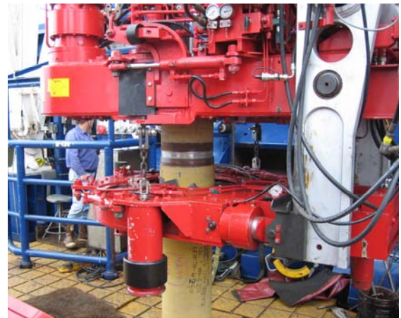
Automated tongs making up a connection
